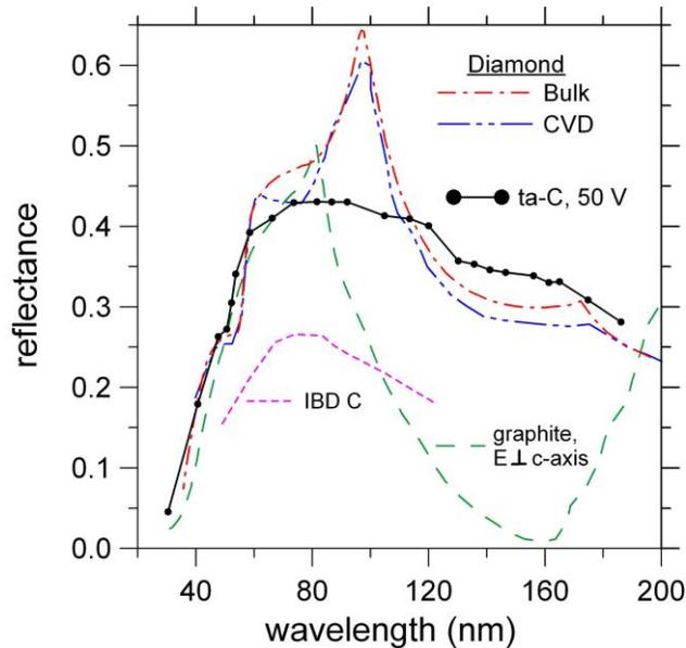
Fig. 2. The EUV-FUV reflectance of a ta-C film compared to other forms of high-reflectance, solid-state C material: bulk diamond [22], CVD amorphous diamond (typical thickness: 15  $\mu\text{m}$ ) [24], graphite (E $\perp$ c-axis) [38], IBD C (24-nm thick) [29].
