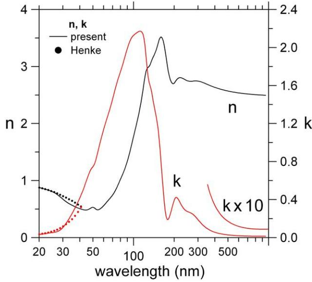
Fig. 5. The optical constants  $n$  and  $k$  of ta-C versus wavelength in log scale. The semi-empirical data of Henke et al. [54] are also shown.
