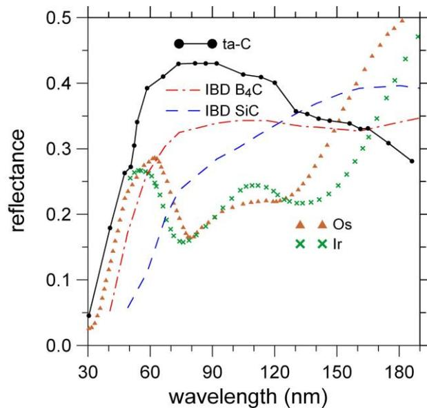
Fig. 3. The EUV-FUV reflectance of a ta-C film compared to other thin-film materials with relatively high reflectance below 120 nm: aged IBD SiC [39], aged IBD B<sub>4</sub>C [40], and evaporation-deposited Ir [41] and Os [42].
