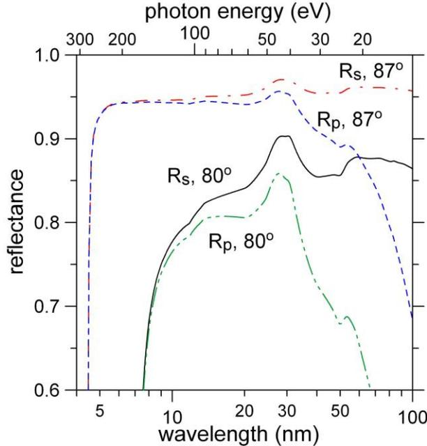
Fig. 6. Calculated ta-C EUV reflectance at two grazing incidence angles measured from the normal versus wavelength in log scale.
