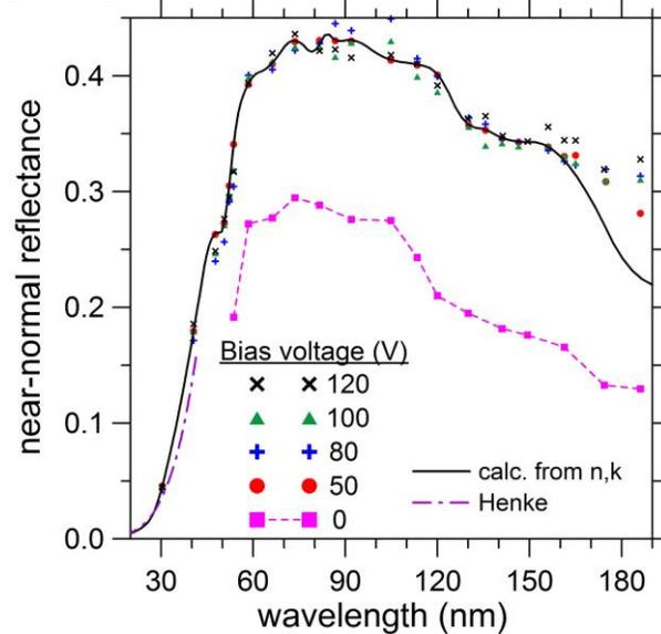
Fig. 1. EUV-FUV reflectance of five C samples grown with the plotted bias voltage as a function of wavelength. The estimated average C ion energy is given in Table 1. Solid line: reflectance calculated with the present optical constants. The semi-empirical data of Henke et al. [54] are also shown.
