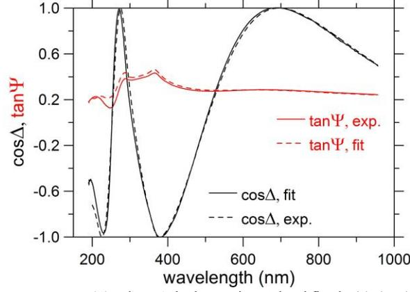
Fig. 4. Ellipsometry parameters  $\tan \Psi$  and  $\cos \Delta$ , both experimental and fitted with the obtained  $n, k$  data, as a function of wavelength measured for the ta-C film deposited with 50-V bias voltage.
