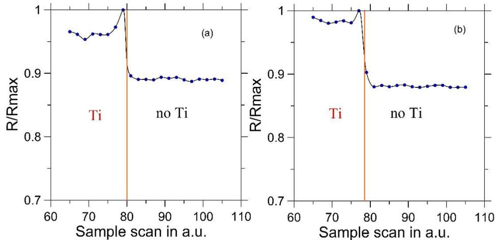
Fig. 2. Normalized reflectance at ~160 nm versus sample scan for Al mirrors with the MgF<sub>2</sub> protective layer deposited at 225 °C (a) and RT (b). One half was pre-coated with a 3-nm thick Ti film and the other half was not pre-coated. A line is plotted to indicate the separation between the seeded and the unseeded areas.
