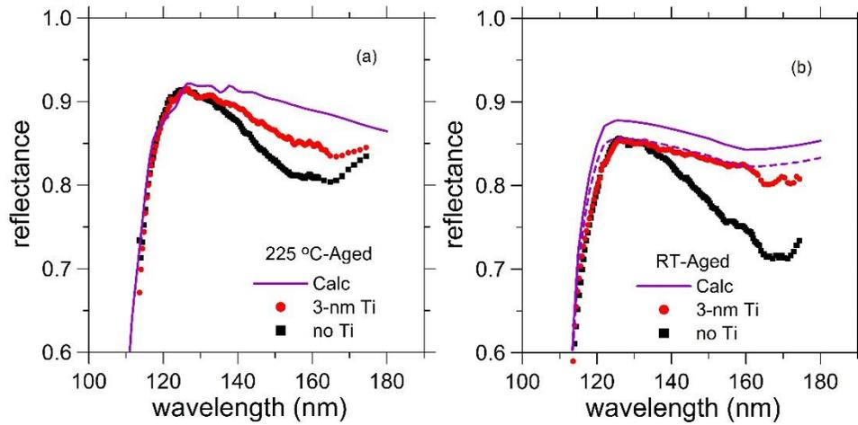
Fig. 1. Reflectance of Al mirrors with the MgF<sub>2</sub> protective layer deposited at 225 °C (a) and RT (b). One half of each mirror was pre-coated with a 3-nm thick Ti film and the other half was not pre-coated. Calc stands for calculated reflectance using the optical constants of Al [18,19] and of MgF<sub>2</sub> deposited either at 250 °C [14] [(a) 25-nm thick] or at RT [20] [(b) 27-nm thick]. Dashed line: reduced calculation (see text).
