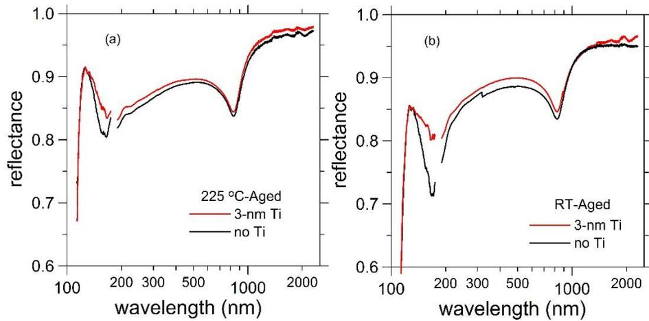
Fig. 4. Reflectance vs. wavelength from the FUV to the IR of Al mirrors with the MgF<sub>2</sub> protective layer deposited at 225 °C (a) and RT (b). One half was pre-coated with a 3-nm thick Ti film and the other half was not pre-coated.
